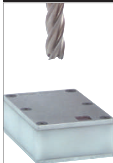
Slowly lower cutting tool toward Tool Setter
