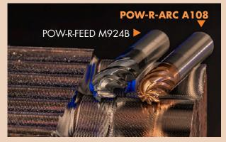
The tools: The POW-R-FEED M924B (left, ¾ in. dia., 4-flute ball end, 1 in. LOC) v. the POW-R-ARC A108 (right, ¾ in. dia., 8-flute ball end, 1 in. LOC) Material: A2 at 60 HRc. Using the same stepover value, the new POW-R-ARC 8-flute tool provides a superior 3D contour cut 5x faster, with barely visible ridges (far right) and very little finish work.
